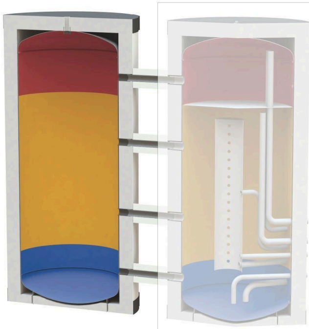
Illustration 15: Connection between Standard and System Storage tanks
